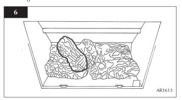
7.5 There are two ash panels which lay across the front of the burner skin. Place the panel with the flat edge facing the left side of the firebox. There are location holes on this log which fit over the screw holes of the burner skin.
